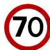
Sign No. RUS 024 to indicate that a motorway speed limit applies
